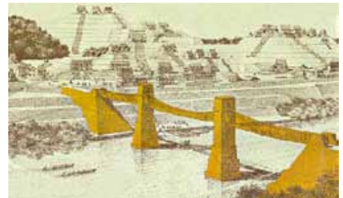
The cables spanned between cast concrete and stone towers topped by Maya arches.
