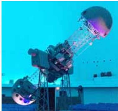
The machine that still functions in the present dome at the Miami Science Museum is a Spitz model STP, or "Space Transit Planetarium"
