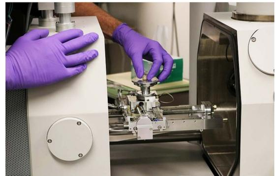
Bead being inserted into the scanning electron microscope chamber in the Optical Properties Lab of the Library of Congress. Photo by Rosemary Ryan.
