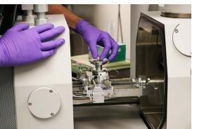
Bead being inserted into the scanning electron microscope chamber in the Optical Properties Lab of the Library of Congress. Photo by Rosemary Ryan.
