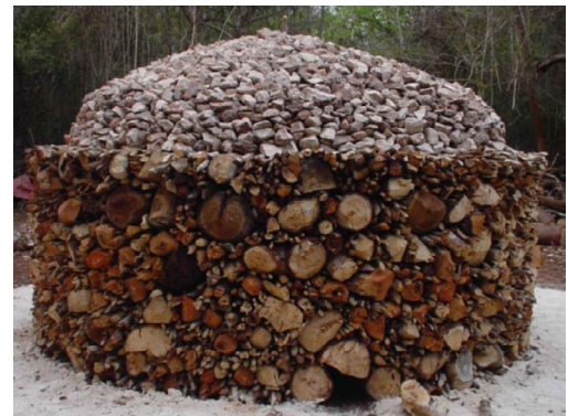
▲ Fig. 4: Experimental burnt lime pyre constructed by Tomás Gallareta Negrón and Rossana May Ciau at Labná.
