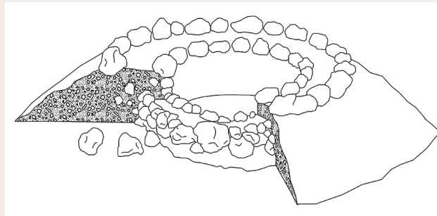
Fig. 5: A diagram of a Pre-Colonial Maya lime pit-kiln from the Puuc Region of the Northern lowlands.
