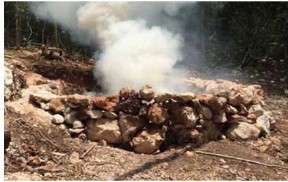
▲ Fig. 2: Lime pit-kiln in use.
